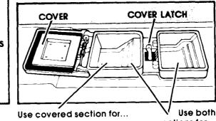
Use covered section for. NORMAL WASH Cycle LOW ENERGY WASH Cycle V Use both sections for... POTS & PANS Cycle HEAVY WASH Cycle
